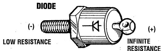
A low resistance should be found with the leads in one direction, and infinite resistance (blocking) in the other direction. Different meters will read different resistance values through the diode.
