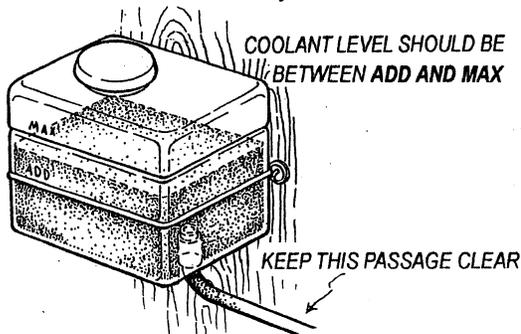
**NOTE:** Periodically check the condition of the manifold pressure cap. Ensure that the upper and lower rubber seals are in good condition and check that the vacuum valve opens and closes tightly. Carry a spare cap.
