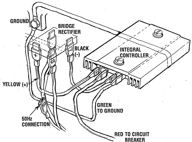
**NOTE:** Should the battery charger or bridge rectifier fail, the generator windings are protected by a 30 amp fuse.
