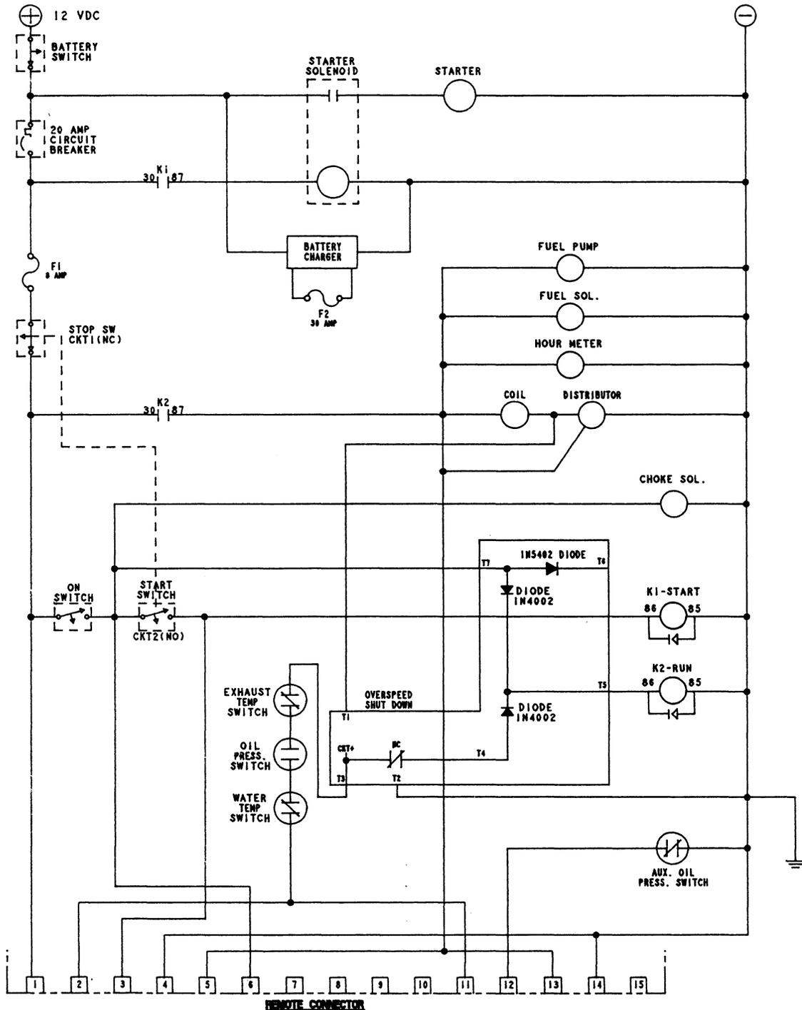
**NOTE:** To by-pass the Overspeed Shutdown for test purposes when troubleshooting, move the connection T3 over to and connect with T5.
