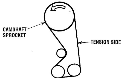
7. Loosen the temporarily tightened tensioner nut on the water pump side 1 or 2 turns, and tension the belt making use of spring force.
