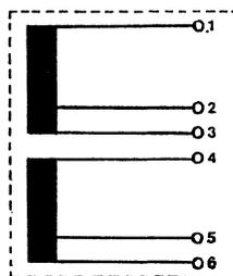
**NOTE:** THE NUMBERED LEADS ON THE TERMINAL BLOCK ARE NOT IN ANY NUMERICAL ORDER. THEY ARE AS SHOWN BELOW
