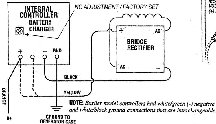
**NOTE:** The battery charging circuit is totally separate from the AC output of the generator. The generator output affects the circuit's output, but not the reverse.
